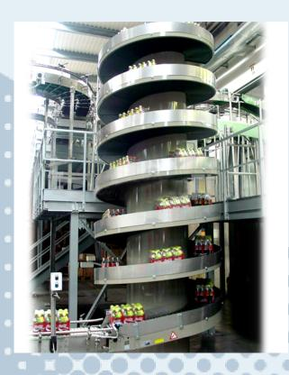
Vertical spiral conveyors are an ideal choice for space savings. They can move lightweight product efficiently, provide merging functionality, and have pick module and product accumulation capabilities.
