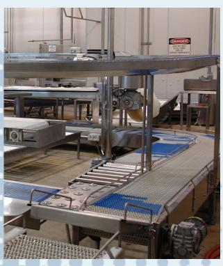
Stainless steel conveyor systems for food, pharmaceutical and other industries provide a corrosion free solution for applications where a wash down environment is required.
