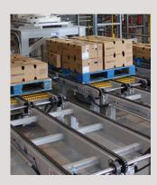
Thomas Conveyor offers a complete line of pallet conveyors for applications within the manufacturing, warehousing and distribution industries.
