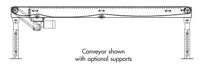
BELTING: 1/2" x 1" x 11 ga. clinched edge, galvanized wire mesh belt.
