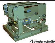
V-belt transters are ideal for medium duty applications and are often used where product could be damaged by strands of chain on heavier duty chain transfers. Unit at left shown with frame cutout for use in belt driven live roller conveyor with 6" wide belting.
