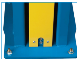
Pallet sensor to detect pallet presence before extending forks
