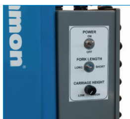
Operator console mounted to back of mast
