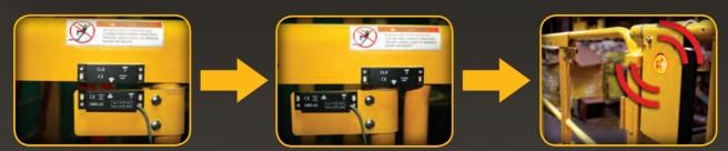
EdgeAlert™ determines when a gate has been opened using dual channel coded sensors.
