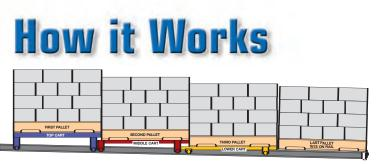
First pallet is placed on the top cart and pushed back. This exposes the next cart for loading. When the second pallet is positioned and pushed back, the third cart is ready. This continues until all the pallet positions are filled. The last pallet sits on the rail itself.
