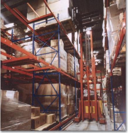
Swing Reach For the ultimate in maximum density and selectivity, combine Glide-In with a Turret Truck in narrow aisle access situations.
