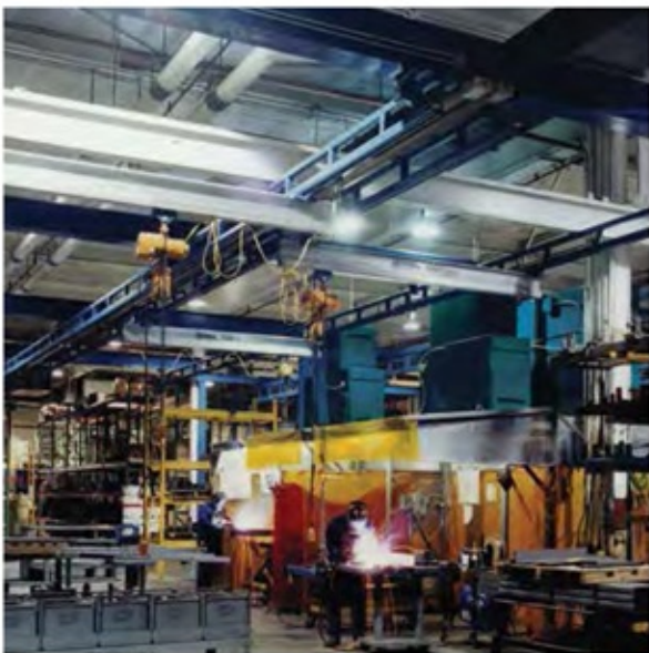
Aluminum Work Station Bridge Cranes
