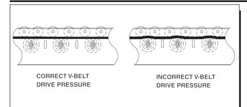
Maintaining proper drive belt pressure is vital to proper unit operation and long V-belt life. Over-applying drive belt pressure requires more horsepower and may harm unit drive and take-up components. Belt life is drastically reduced when unit is operated with incorrect drive belt pressure.
