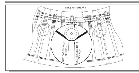
Maintaining proper belt tension is vital to proper unit operation and long V-belt life. Over-tensioning drive belt requires more horsepower, decreases belt life and may harm unit drive and take-up sheaves.
