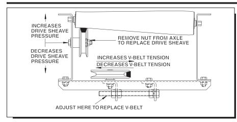
As outlined in previous sections, the importance of properly setting drive tension and drive pressure on V-belts simply cannot be overstated. When V-belt or drive sheaves are out of adjustment, life of sheaves and V-belting may be drastically reduced, thus requiring untimely replacement(s).
