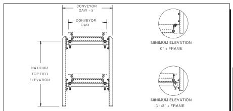
NOTE: To install, raise conveyor to desired elevation, place cross pipe underneath lower conveyor flange, attach cross pipe to upright legs and use U-shaped retainer ("hat") bracket to connect cross pipe to lower conveyor flange.
