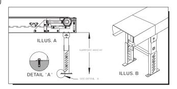
Supports are normally shipped at minimum support height.
