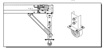
Knee braces are most commonly used at the terminal ends of long runs of conveyor lines and are recommended on inclined (or declined) floor-to-floor belt conveyors for added stability.
