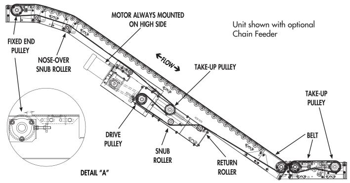
CAUTION: If pulleys are adjusted during installation or maintenance, it is crucial that nip point guards (at both ends of conveyor) are readjusted. See DETAIL"A" at left. Center drive guards MUST be replaced after installation or maintenance. If optional feeder is used, nip point guards in end assemblies (including drive or fixed end pulley) must be adjusted when feeder pulleys are adjusted.
