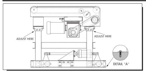
CAUTION: Always anchor permanent supports to floor (or mounting surface). Use 3/8" x 2-1/2" (or longer) wedge anchors for permanent installation in concrete flooring (see detail "A").
