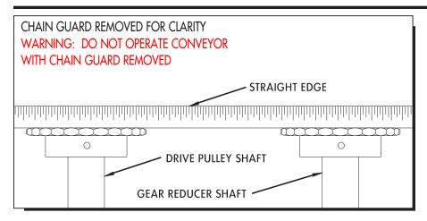
WARNING: To check drive sprocket alignment, it is imperative that conveyor is shut "OFF" and power source is locked out before any adjustments are attempted.
