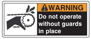
ABOVE: Label attached to all protective guards (drives, roller guards, etc.)
