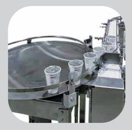
Rotary tables enable the collation and accumulation of products from conveyor lines and packing areas creating a buffer zone on a low speed line and also providing accumulation at the end of a production line. Ideal for areas that are not large enough or not suitable for an automated system.
