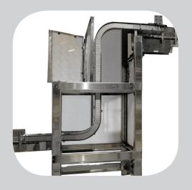
Standard speeds of up to 200 feet per minute can be expected on the MCE side gripper elevator. The side gripper elevator adjusts from 0" - 14" wide with the turn of a single handwheel and is designed to quickly change the elevation of various bottles, jars, cans, containers, and packages.
