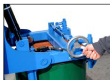
1. Manually secure clamp to grip drum
