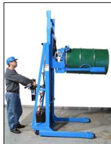
4. Manually release clamp, then raise drum to place in rack
