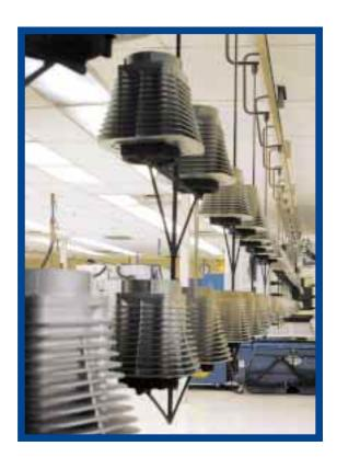
Inverted Conveyors offer clean operation with uniquely designed flexible vertical pendants.
