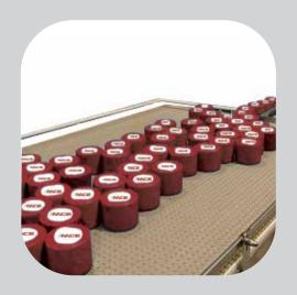
The Re-Flow Accumulation Table is best used as an in-line accumulation solution that requires single-file discharge. The accumulator can handle round and non-round containers. It provides random delivery of products to downstream operations.
