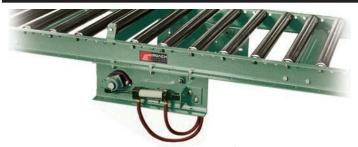
Pneumatic gravity conveyor stops are used where automatic line control is required such as slug accumulation, indexing, etc. This stop is designed for 3-1/2" and 4" deep frames.
