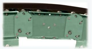
Nose-over brackets may be attached to slider bed or roller bed belt conveyors to smoothly bridge the transition of inclined or declined bed sections to horizontal bed sections. NOTE: 1-foot bed section supplied on double nose-
