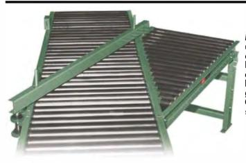
Manual diverters are used to divert packages off of a main conveying line onto other conveyors. Diverter can be used on powered or gravity conveyors. Conveyors shown are optional.
