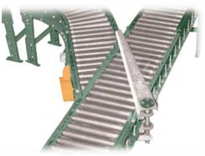
Pneumatic diverters are used to divert packages off main conveyor line onto spurs. This diverter may be utilized in powered or gravity conveyor applications. Conveyors shown are optional.
