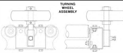
Turning wheel and turning post assemblies (turning post shown lower right) are commonly used in applications with converging or diverging spurs. These simple transition devices assist products with smooth transition to or from spur line.
