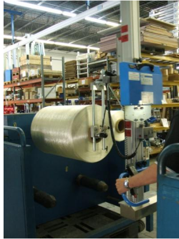
Roll Handling-Squeeze-O-Turn™ Core Vertical to Cores Horizontal
