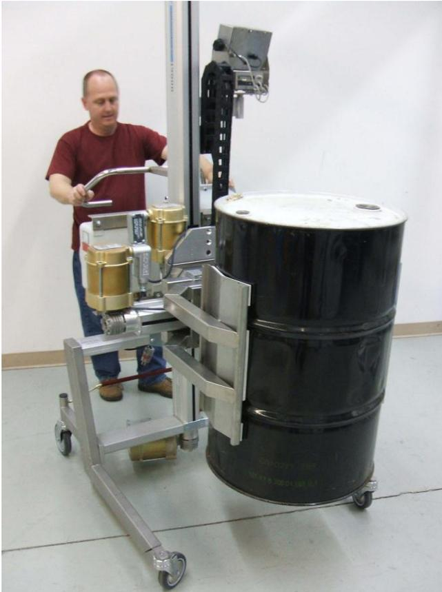
The 19000 EEx d Series Explosion Proof lifter offers users the flexibility to meet the demands of explosion proof material handling needs combined with ergonomic lifters. The lifter is self-contained and has Explosion Proof enclosures for the control panel, Power Pack (batteries) w/Charger along with motor(s) according to the requirements as noted in the “Certificates of Compliance as noted below.
