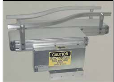
Side transfer from belt to belt.
