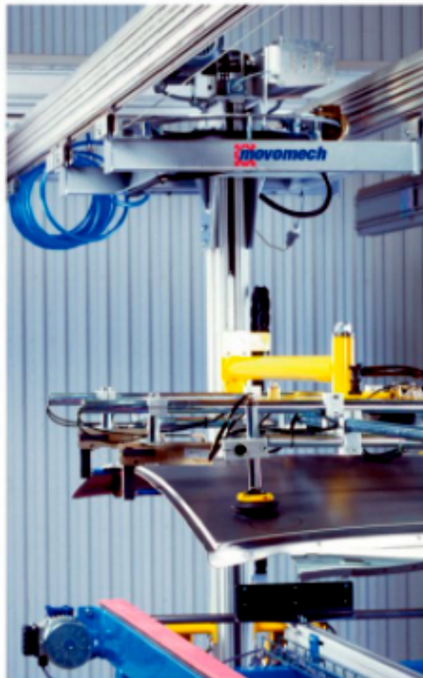
Sheet metal handling with Mechstick E and vacuum gripper
