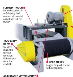
ADJUSTABLE MOTOR MOUNT Heavy-duty motor mount designed to fit a variety of motors. Adjustable for V-belt tensioning. Available with three phase or single phase motors, TEFC or explosion proof.
