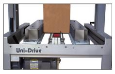
Reliable and Repeatable Performance Wexxar/Bel's exclusive Uni-Drive System synchronizes both side belts, eliminating case skew, ensuring a square seal even after extended periods of use.
